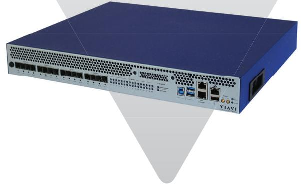
The Xgig 4K16 is a single platform that allows for simultaneous protocol analysis and error injection for PCIe 4th generation protocol traffic at all layers of the stack. It supports Lane Widths of x1, x2, x4, x8, and x16 at Link Speeds of 2.5 GT/s, 5.0 GT/s, 8.0 GT/s and 16 GT/s.
